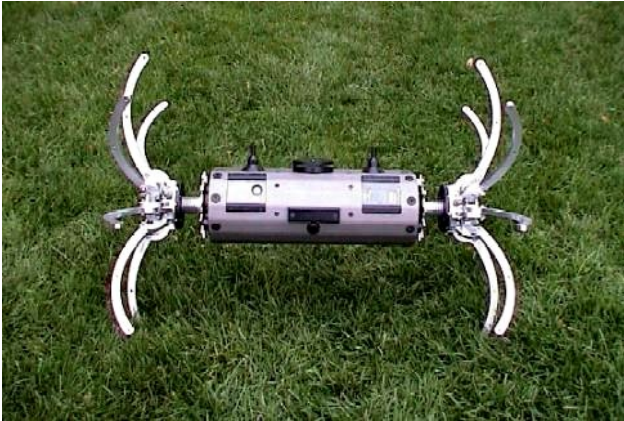
Figure 4: The actuated-wheel MegaScout shown with its wheels retracted and expanded.
