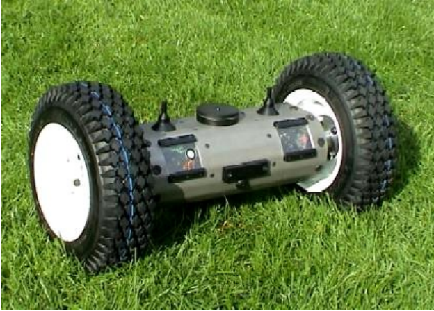
Figure 3: The MegaScout equipped with balloon tires.
