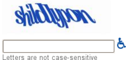
Figure 2.5: A sample CAPTCHA, shown to a user as part of the account signup process for creating a Google Mail (Gmail) account.
