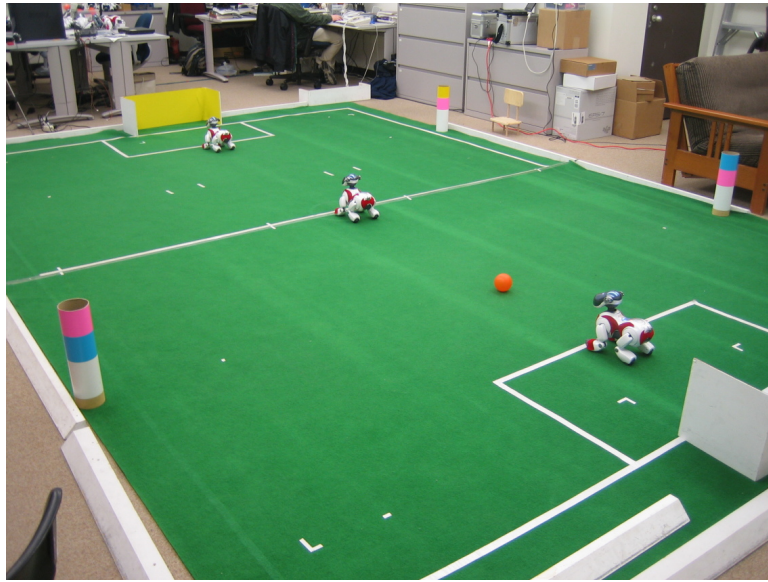
Figure A.5: Initial position for each experimental trial. The three robots are placed in three positions on the field, with the ball in the defense area. The experiment proceeds until the robots advance the ball past the end line of the opposite half of the field.
