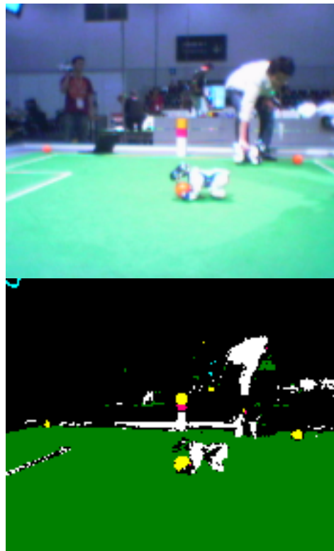
Fig. 4. An example of a raw image from the robot’s camera (top) along with the corresponding color segmented image (bottom), used for object detection. In the images, an AIBO robot in a blue uniform holds the ball under its chin in preparation for a kick. A localization marker, consisting of two colored bands on top of a white column, is visible at the edge of the field.
